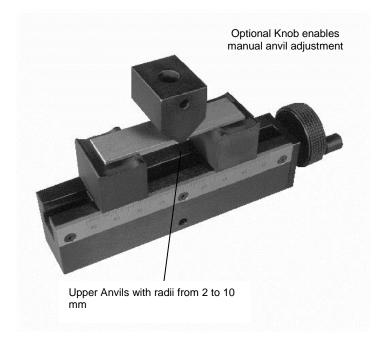
For flexural and fracture toughness bond tests including determination of flexural modulus, flexural strength and flexural yield strength. The G103-3 three point fixture can be modified with an optional conversion kit to provide four point bending.
