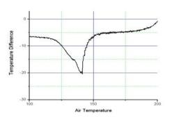
The temperature difference between the air and the sample is not zero but close to  $-6^{\circ}$ C under these conditions. The plot above has been zoomed to illustrate the onset of exothermic reaction, clearly close to  $170^{\circ}$ C. The onset seen from a derivative temperature plot is not precise. The plots shown below indicates onset near  $180^{\circ}$ C.
