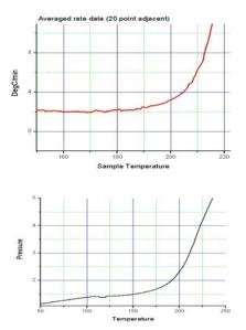
Pressure data plotted against temperature is also a good indicator of reaction—here without any solvent in the sample a reference is less relevant. Note the discontinuity at the melting. The graph shown above indicates the pressure rise and shows onset near  $160^{\circ}$ C,  $10^{\circ}$ C lower than the thermal data.
