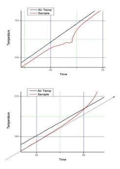
The graphs highlight the melting endotherm and the decomposition exotherm.
