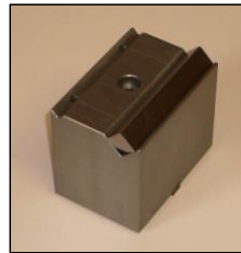
J22 Milled or machined knife edge 'roller'.
