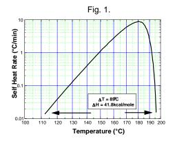
close to 42 Kcal/mole and thus this data shows very good agreement and hence the adiabaticity of the Accelerating Rate Calorimeter. Indeed this is a test which could be done to verify performance of the Accelerating Rate Calorimeter or to compare it with other calorimetry devices.
