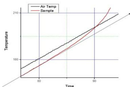
The graphs highlight the melting endotherm and the decomposition exotherm.
