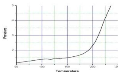
Pressure data plotted against temperature is also a good indicator of reaction—here without any solvent in the sample a reference is less relevant. Note the discontinuity at the melting. The graph shown above indicates the pressure rise and shows onset near  $160^{\circ}\text{C}$ ,  $10^{\circ}\text{C}$  lower than the thermal data.
