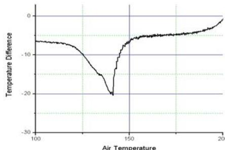
The temperature difference between the air and the sample is not zero but close to  $-6^{\circ}\text{C}$  under these conditions. The plot above has been zoomed to illustrate the onset of exothermic reaction, clearly close to  $170^{\circ}\text{C}$ . The onset seen from a derivative temperature plot is not precise. The plots shown below indicates onset near  $180^{\circ}\text{C}$ .
