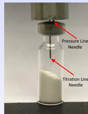
Standard crimp top sample vials with natural rubber PTFE faced septa lid hold pressure up to 5bar.
